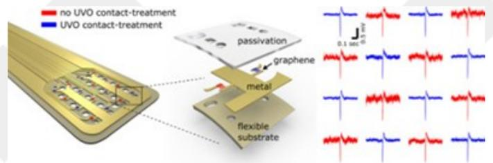
Graphene transistors provides unique capabilities for recording high fidelity DC-coupled neural recordings, this capability enable the study of the role of the infra-slow activity in the brain behavior and its pathologies. Recent research has provided better knowledge on electrical modeling and fabrication process, increasing the maturity of this novel technology.
