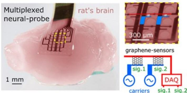
The connectivity is one of the major limiting factors in the development of high density neural interfaces. The use of graphene graphene transistors arranged in addressable arrays enable the use of multiplexed read-out strategies to reduce the connectivity footprint. Recent developments demonstrated the capability of GFETs based arrays for implementing Time Domain
