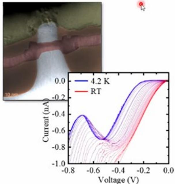
The aim of the IONS4SET project (Ion-irradiation-induced Si nanodot Self-Assembly for Hybrid SET-CMOS Technology) was to create single electron transistors for ultra-low power electronics so that the component using these optimized transistors delivers good performance at very low energy consumption. This
