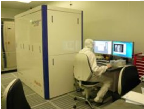
Electron beam lithography system
