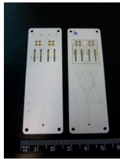
Multiplexed chip (top and bottom view) (Arcatech4-CAJAL4EU project)
