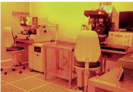
Mask aligners for microsystems ("non-CMOS") photolithography.
