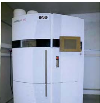
Rapid Manufacturing with an EOS Formiga P100 laser sintering system.
